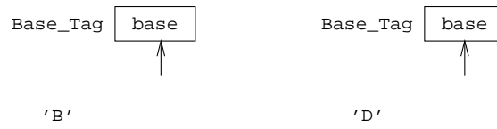
Figure 3.13 The two dependency graphs of Base_Tag .
